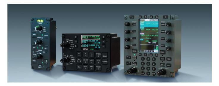
Control panel is designed as the control and indication unit for remote control of the radio equipment.
