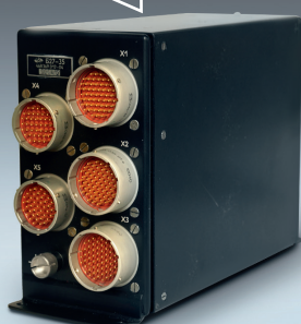
Amplifying and switch unit B27-35 with DSP and SELCAL
